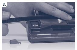
Then gently remove the brush by holding a length of bristles and sliding it out. Once replaced please remember to replace the yellow insert.
