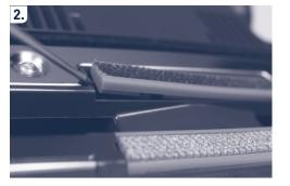
Remove the red, flat thread lifters by inserting a narrow-bladed screwdriver into the indentations on either side and gently prising up the inserts.
