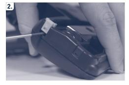
Now gently ease out the yellow locking insert with a narrow screwdriver.
