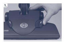
To make the brush strip easier to grasp, push the 'down' foot switch to lower it.
